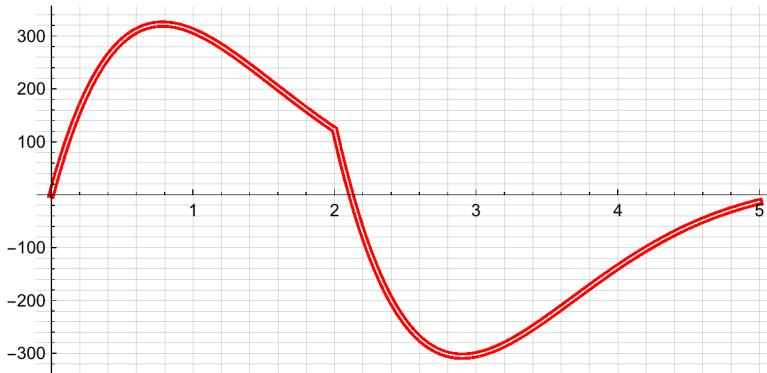
The following plot shows the interpolating function (same as plot p6) along with the text answer (p7). It can be seen from the plots that the interpolated solution follows the exact (Laplace) solution closely.
